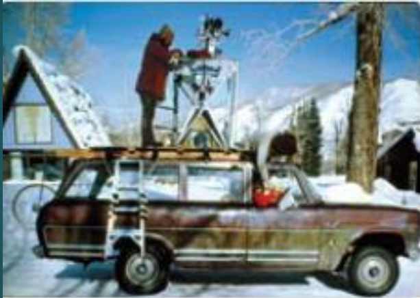
Aspen Movie Map camera vehicle, ca. 1978 Credit: MIT Architecture Machine Group
